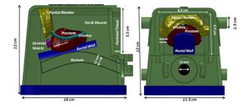
Internal tissues setup of the prostate phantom End fire model.
